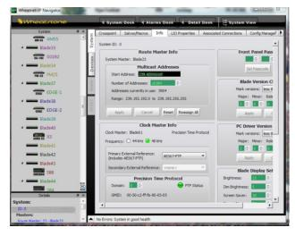
Finding #4. When adding an AES67 device to the network, pay attention to packet timing incompatibilities. WheatNet-IP uses 1/4 ms packet timing for minimum latency. Most AES67 devices also support 1/4 ms packet timing but some, such as Dante, do not. For those devices that do not use 1/4 ms packet timing, we enabled the AES67 1 ms Support option in WheatNet-IP Navigator, as shown below.
