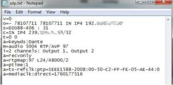
Above are a few sample SDP files from WheatNet-IP and Dante showing multicast address, packet timing, sample rate and stream formats.
