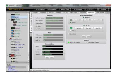
Finding #5. Some AES67 devices do not offer an easy way to manually manage streaming details, although these devices often can ingest these details in the form of an SDP file. In our case, we created SDP files by simply right-clicking on the desired source stream's name in the Navigator crosspoint grid and opening a window that let us create the file.
